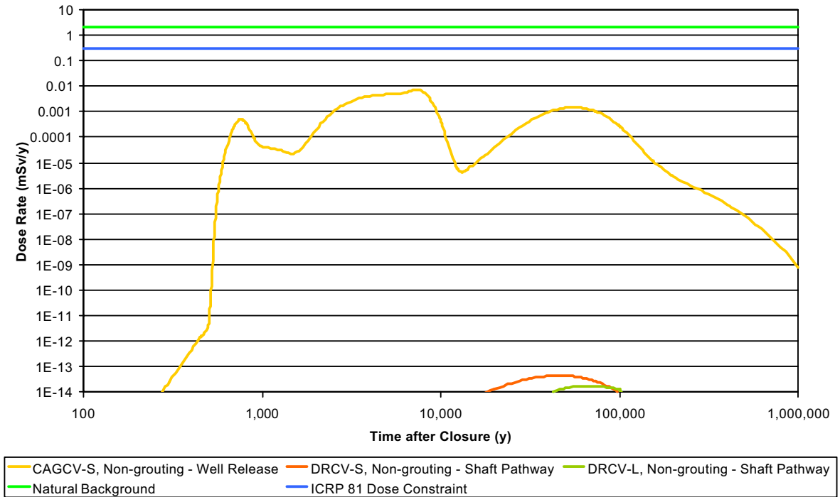
Figure 7: Calculated Dose Rates for the Most Significant Calculation Cases for the CAGCV and DRCV Concepts, Reference Scenario
